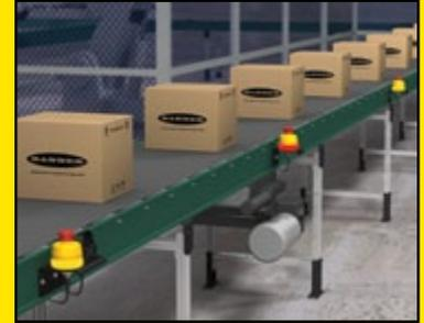
When 30 mm mount E-Stop buttons are wired in series, the built-in logic function allows for clear indication of which device has been pushed.
