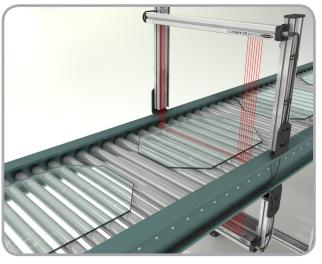
A specially-designed EZ-ARRAY detects glass plates for profiling and broken edge detection. The receiver is customized with low-contrast detection to successfully see clear objects.
