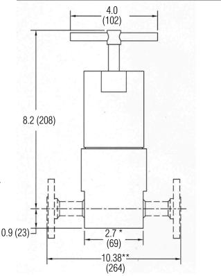
\* 1/2" THD, FSW, & BWE Ends, weight 30 lbs (13,6 kgs) \*\* 1/2" Flanged End, ANSI 2500#, weight 45 lbs (20,5 kgs)
