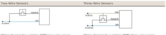
Wiring diagram for a sinking (NPN) two-wire sensor powered using the SureCross device terminal block. Under certain conditions, the dc commons between the sensor and the SureCross device might need to be connected.
