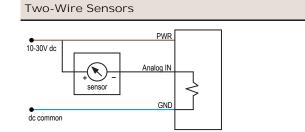
Two-wire analog sensor powered from a 10–30V dc power SureCross device using the PWR terminal.
