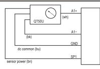
Four-wire QT50U sensor, using a FlexPower Node, and powered using the Node's switch power terminal. The QT50U output is set to 4–20 mA.
