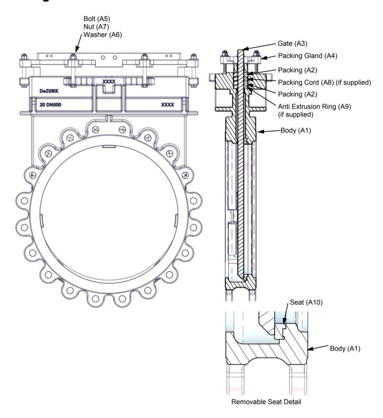
Figure 2—Component Identification
