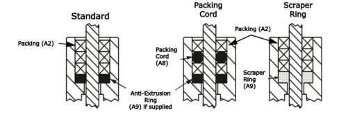
Figure 3—Packing Ring Detail
