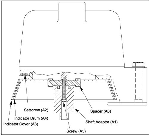
Figure 4 - Indicator Adjustment Components
