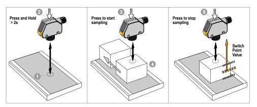
**Note:** The sensor must be set to  $\frac{1}{2}c^{\frac{1}{2}} = \frac{1}{2}c^{\frac{1}{2}}$  to use the following instructions. The DYN indicator is amber to indicate Dynamic TEACH mode.
