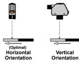
Figure 11. Orientation for highly reflective target
