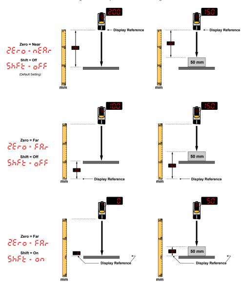
Figure 14. Example Zero and Shift settings
