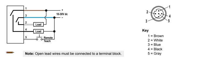
Note: The input wire function is user-selectable. The default for the input wire function is off (disabled).
