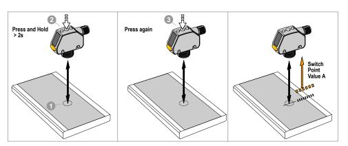
**Note:** The sensor must be set to  $\frac{1}{5}c^{h} = \frac{1}{5}c^{5}$  to use the following instructions. The BGS indicator is amber to indicate Background Suppression mode.
