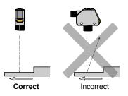
Figure 10. Orientation for a color or luster difference
