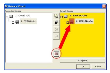
The "Show Device" option is particularly useful after the Net-Autoset procedure or whenever it is necessary to physically identify a specific scanner on the network. Indeed, it activates the following signals which physically indicate the scanner corresponding to the one selected, in particular:
