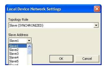
SYNCHRONIZED: The Master SYNCHRONIZED / Slave SYNCHRONIZED configuration is the traditional ID-NET™ network configuration in which the On-Line Operating Mode is used.
