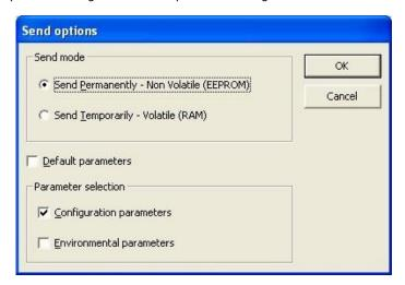
Environmental Parameters regard the scanner Identity and Position in a Network (ID-NET™, Master/Slave RS232, MUX 32) and <u>are not influenced</u> by the Send Default and Send Configuration commands. This allows individual scanners to be configured differently without affecting their recognized position in the network.
