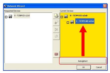
a. if the <u>slave scanners</u> have already been configured and <u>wired</u> to the network, click on the Autodetect button to start a polling procedure of the current network. The master and all slave scanners found will be represented in the "Current Devices" area. Then, select the desired slave
