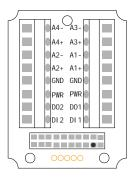
Ax+ and Ax-. Analog IN x. Analog inputs for devices requiring more than one connection, such as thermocouples or RTDs. When there is no Ax-, use Ax+ as an analog input.
