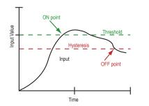
In the example shown graphically, the input is considered on at 15 mA. To consider the input off at 13 mA, set the hysteresis to 2 mA. The input will be considered off when the value is 2 mA less than the threshold.
