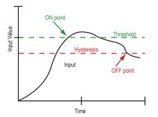
In the example shown graphically, the input is considered on at 15 mA. To consider the input off at 13 mA, set the hysteresis to 2 mA. The input will be considered off when the value is 2 mA less than the threshold.
