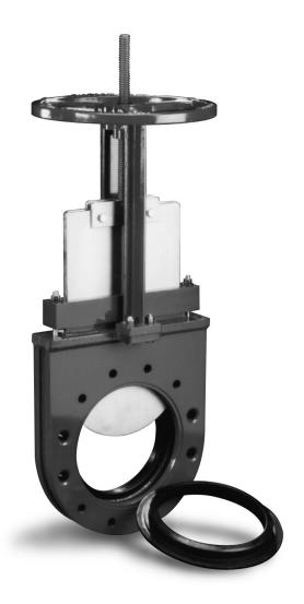
The Red Valve Series D Flexgate Slurry Knife Gate Valve is a 100% full bore, truly bi-directional valve designed for tough slurry applications. The Flexgate features heavyduty elastomer seat cartridges which provide droptight closure and are replaced <u>WITHOUT ANY VALVE DISASSEMBLY</u>, for ease of maintenance.
