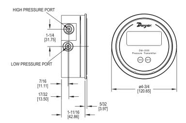
The **Dwyer Series DM-2000 Differential Pressure Transmitter** senses the pressure of air and compatible gases and sends a standard 4-20 mA output signal. The DM-2000 housing is specifically designed to mount in the same diameter cutout as a standard Magnehelic® differential gage. A wide range of models are available factory calibrated to specific ranges.
