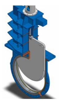
The standard knife gate valve has a rounded gate edge and the discharge flange is the same size as the inlet flange.
