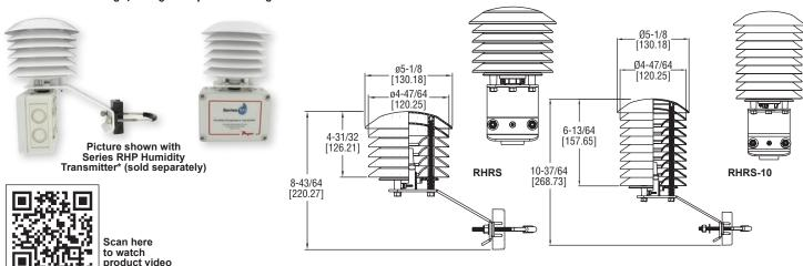
The **SERIES RHRS** Radiation Shield protects outside air humidity transmitters from rain and radiated heat. With the curved shape and color of the plates, air flow is able to move across the sensor to keep radiated temperatures from rooftops and surrounding surfaces from affecting humidity readings.
