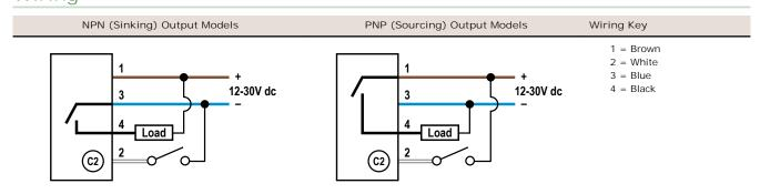
Cabled wiring diagrams are shown. Quick disconnect (QD) wiring diagrams are functionally identical.
