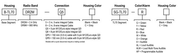
Select the 5-pin base for tower light configurations of up to three modules. Select the 8-pin base for tower light configurations of up to six modules, or when the event counter will be enabled.
