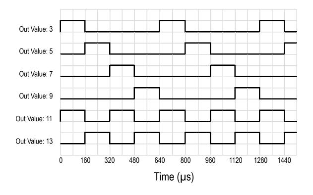
Example -- Lights Racing Up the Stack To program all four lights to come on at a different time to appear to race up the light stack, write a 3 to M1, 5 to M2, 7 to M3, and a 9 to M4.
