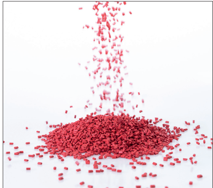
Fig. 2: Plastic granulate for injection molding or extrusion
