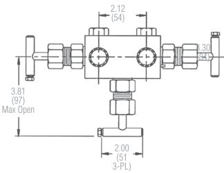
Orifice Size: 0.19" (shutoff); 0.16" (equalizer) Weight: 7.5 lbs (3,4 kgs)
