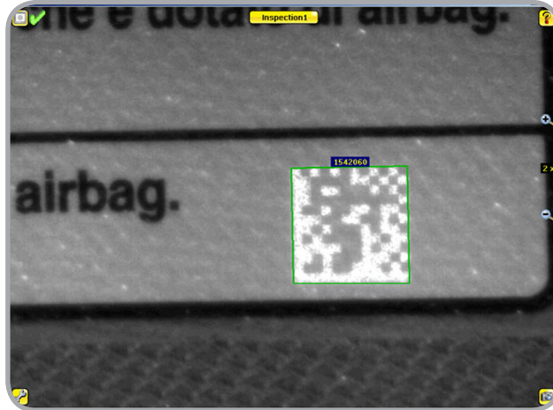
The iVu Plus BCR sensor detects a 2D Data Matrix UV barcode printed on an automotive warning label.
