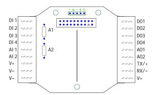
RX/-. Serial communication line for the Gateway. No connection for Nodes
