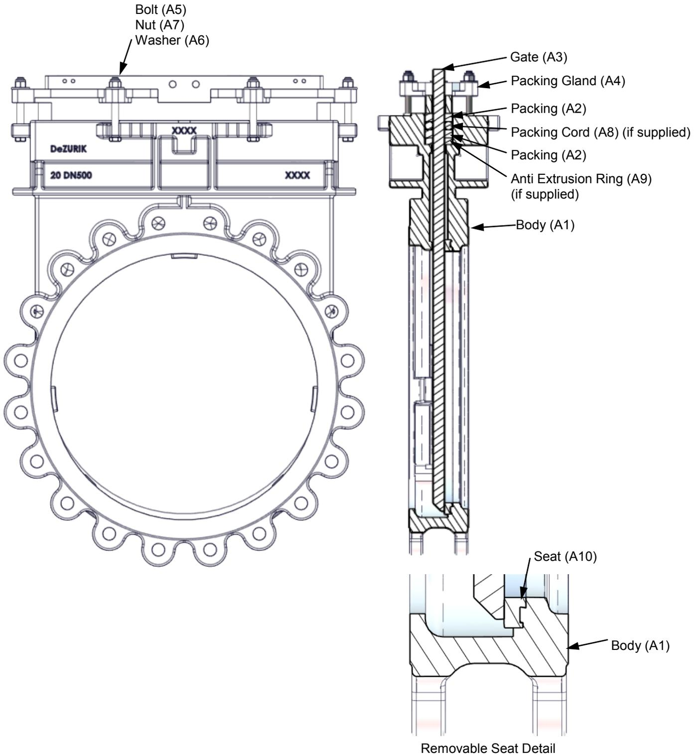
**Figure 2—Component Identification**
