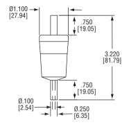
Remove 99.99% of unwanted particles from within your gas flow with the **MODEL F195** Disposable In-Line Filter. Encapsulated microfiber filter elements are able to filter particles as small as 0.1 micron. Filters are completely disposable — simply remove the filter from your line and throw it away when it becomes dirty. The transparent nylon housing makes it simple to determine if the filter needs to be changed.
