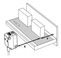
Figure 4. Background Suppression Mode Application Example
