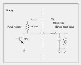
Option 2: Enable the Input Pullup in the iVu TG software (Main Menu > System > Discrete I/O > Input Pullup).
