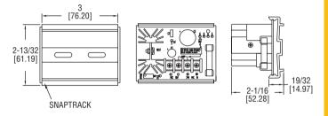
The **MODEL BPS-005** Low Cost DC Power Supply is a regulated .5 A power supply that accepts 24 VAC input and provides an adjustable 1.5 to 29 VDC output. Output voltage adjustments are made using the on-board potentiometer while measuring the output with a multimeter. A compact snap track design allows the power supply to be surface mounted within a panel.
