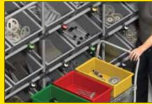
Operators pick parts from bins with yellow, green or red lights and press a button to indicate the job is complete while placing parts in corresponding bin colors.
