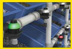
A 2-color K30L lights green to indicate which parts to pick and lights red to indicate an empty bin. A worker presses the button to verify a correct pick.
