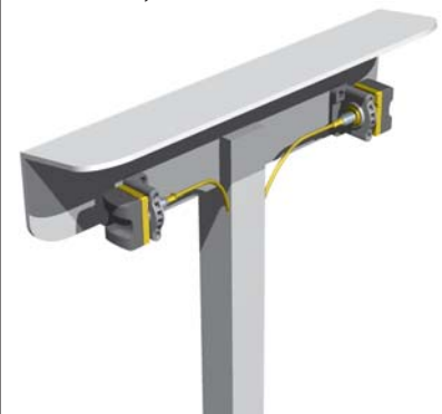
Figure 4. Install STB Buttons so that they are protected to prevent defeat or inadvertent actuation
