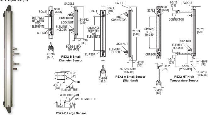
The **SERIES PSX2** Portable Ultrasonic Flowmeter Detectors is paired with Series PUX and PUX2 converters in order to utilize the transit-time difference for measuring flow rates in pipes from the outside.
