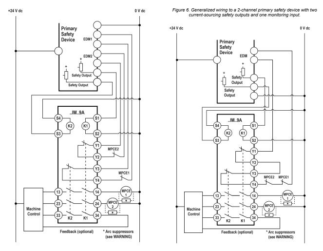
These wiring diagrams are labeled ..IM..9A. The wiring for model ..IM..11A is similar, but not identical because of the different contact arrangement.
