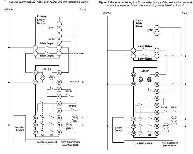
Figure 3. Generalized wiring to a 2-channel primary safety device with two hardcontact safety outputs (FSD1 and FSD2) and two monitoring inputs.
