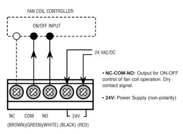
Figure 3 Wiring the Sensor
