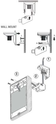
Figure 2 Mounting the Sensor
