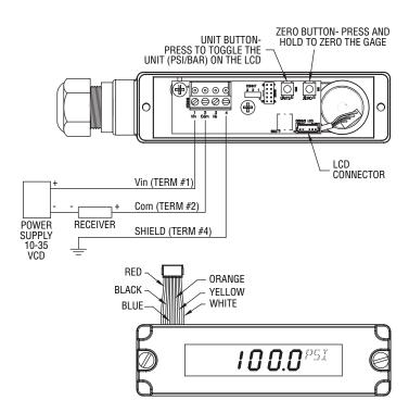
Figure 2: Current Output with Optional LCD
