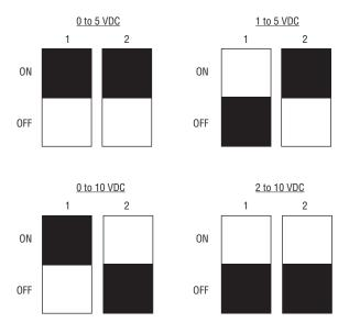
Figure 4: Voltage Output DIP Switch Selection
