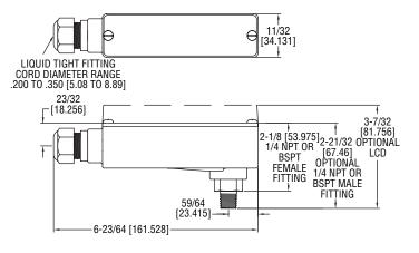
The **SERIES 626 AND 628** Pressure Transmitters monitors the pressure of compatible gases and liquids with 0.25% FS accuracy for 626 models or 1.0% FS accuracy for 628 models. The design employs a pressure sensor that can convert a single positive pressure into a standard 4 to 20 mA output or field selectable voltage output. The terminal block, as well as a zero adjustment button, are easily accessed under the top cover. The Series 626 and 628 are designed to meet NEMA 4X (IP66) construction.
