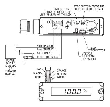
Figure 6: Voltage Output with Optional LCD
