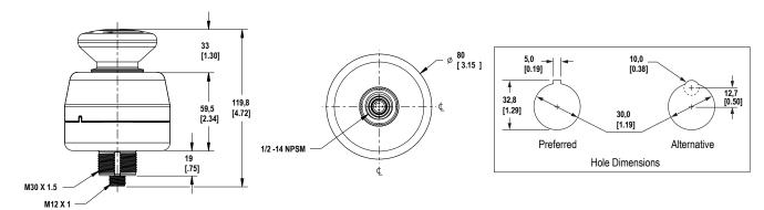
Figure 3. Large 60 mm Pushbutton
