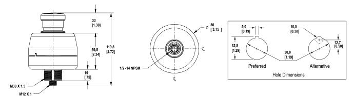
Figure 2. Standard 40 mm Pushbutton
