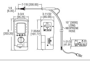
The MODEL 1207A Handheld Flue Gas Combustion Analyzer allows users to monitor four parameters simultaneously and change the parameters shown using the rotary dial selection switch. The unit's memory stores up to 255 time stamped test sets and can output the measurements to a serial printer. For extra protection, the analyzer comes standard with a protective boot and magnetic back.
