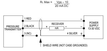
Figure A: Current output connection
