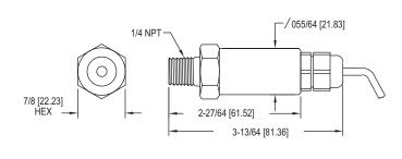
The Series 626 & 628 Pressure Transmitters converts a single positive pressure into a standard 4 to 20 mA output signal. The Series 626 and 628 can be used to accurately measure compatible gases and liquids; Series 626 full scale accuracy is 0.25%; Series 628 full scale accuracy is 1.0% (see specifications). Designed for industrial environments with a NEMA 4X (IP66) housing, this transmitter resists most effects of shock and vibration.
