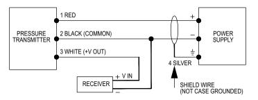
Figure G: Voltage output connection
