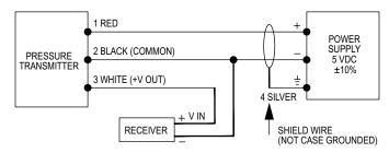
Figure K: Voltage output connection
