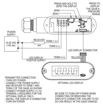
Figure B: Current output with optional LED display connection
