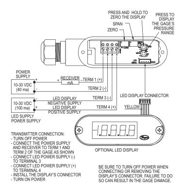
Figure C: Current output with optional LED display using two power supplies
