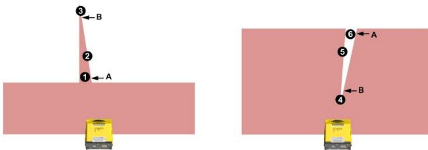
Figure 3-4. Example of inward and outward cone-shaped fields
