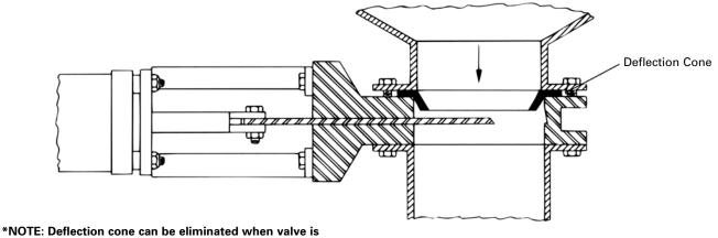
installed with seat upstream on some dry solids service. Contact DeZURIK for assistance.
