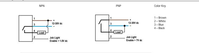
Note: Cabled wiring diagrams are shown. Quick disconnect (QD) wiring diagrams are functionally identical.
