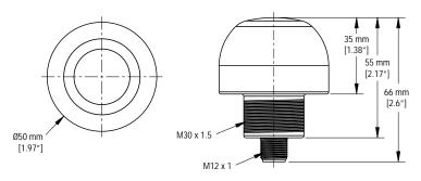
All measurements are listed in millimeters [inches], unless noted otherwise.
