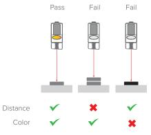
Inspections use distance to verify parts presence and position, and intensity to verify correct color
