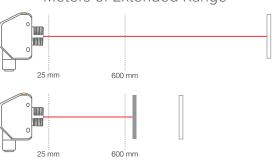
Teach a reference target, even past the maximum measuring range, to detect changes in contrast for presence and absence detection
