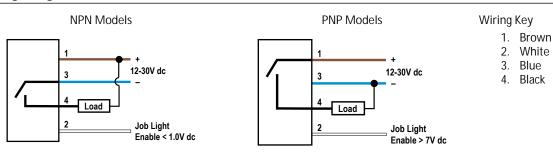
Note: Cabled wiring diagrams are shown. Quick disconnect (QD) wiring diagrams are functionally identical.
